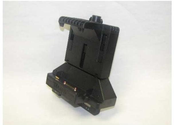
2. Push downward on the wing turn latch until the slide plate is holding the computer in place, then turn the latch to hold the slide plate in the downward position. (See Figure 3)
