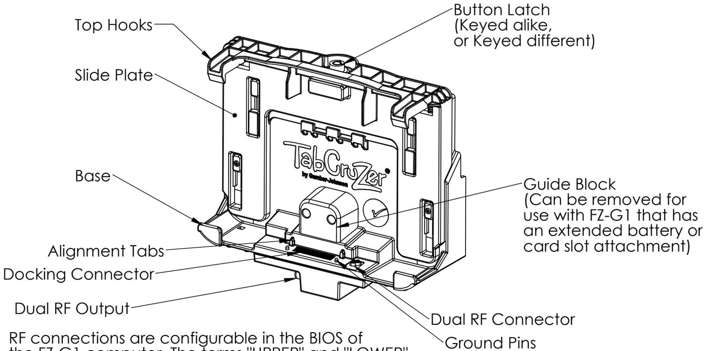
RF connections are configurable in the BIOS of the FZ-G1 computer. The terms "UPPER" and "LOWER" position used in the BIOS of the FZ-G1 computer correlates with Gamber Johnson FZ-G1 Docking Station "Ant 1" and "Ant 2" as follows: "UPPER" = "Ant 1" and "LOWER" = "Ant 2".
